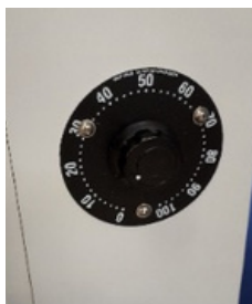
SETTING THE HEATING POWER FROM 0 % TO 100%
